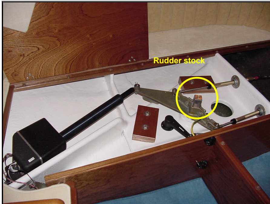
Picture 12 – Rudder stock and automatic pilot linear driving unit
