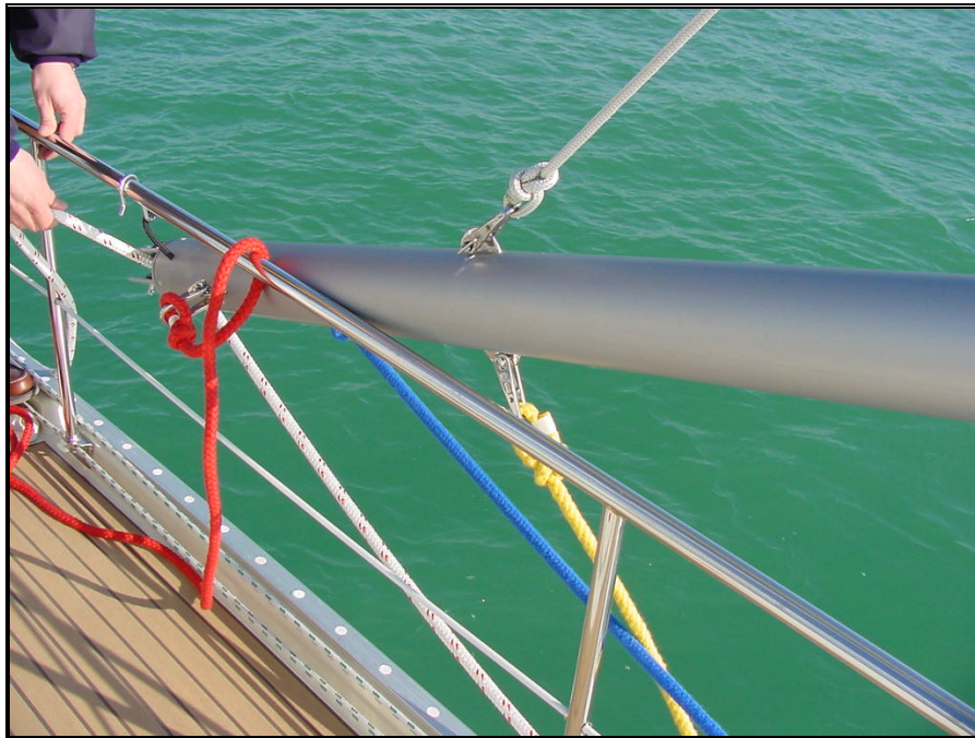
Picture 33 – Attachment of the lines on the pole and way of jib's sheet
